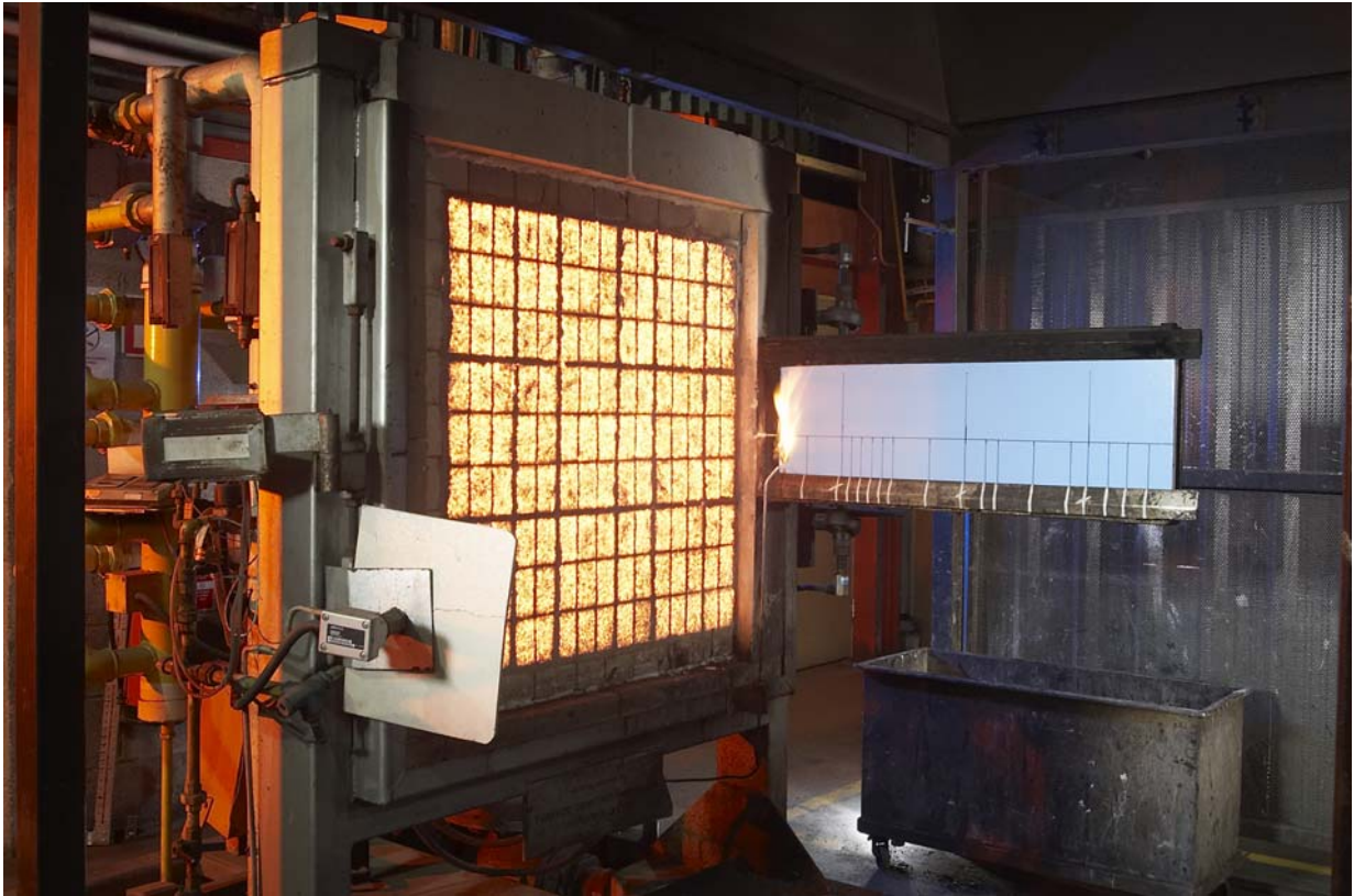
Figure 1. Testing construction materials at Bodycote Warringtonfire UK to BS 476 Parts 6 & 7 – Propagation of flame when in contact with a 500 °C wall of fire. In order to meet a standard materials cannot burn pass the first marker.
