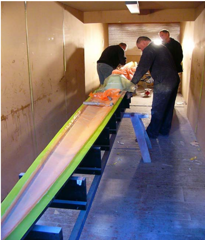
Figure 4 - Image of a Grid Link Wind turbine blade being manufactured using Auspreg UV
