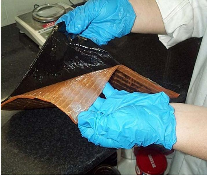
***Figure 4 – The Auspreg UV being taken out of its protective layers prior to applying it into the moulds.***
