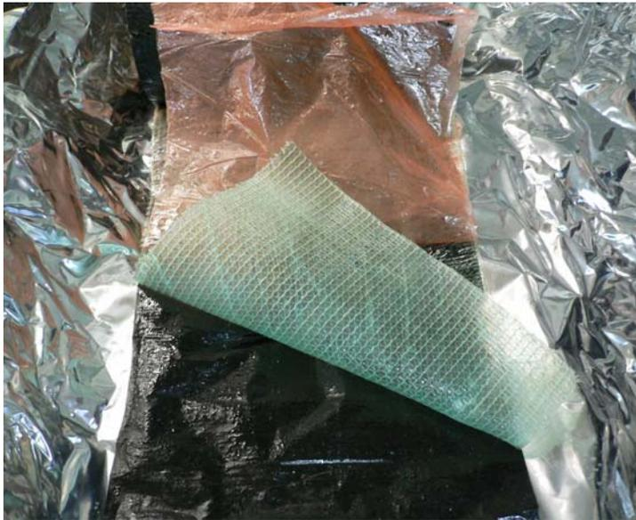
***Figure 5 – Auspreg UV is supplied in rolls 20-30 kilos. In this particular project, the roll lengths were 15m x 1.27m which enabled long train parts to be manufactured with ease.***
