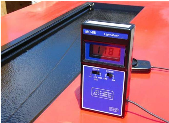
***Figure 2 – A light meter was used to determine whether the products would be cured outside using natural light or inside using metal halide lights.***
