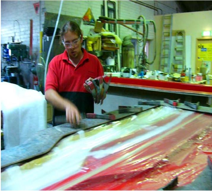
***Figure 6. – A technician clamps down a cover to create an airtight seal during vacuum bagging***
