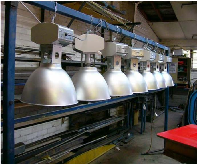
***Figure 3. – Standard metal halide lights or mercury vapour lamps are used were set up for curing the train parts indoors.***
