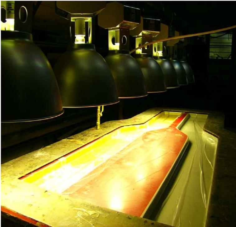
***Figure 7. Lighting in the 360-420 Nm visible light range is applied via a 1000w commercially available metal halide lighting***
