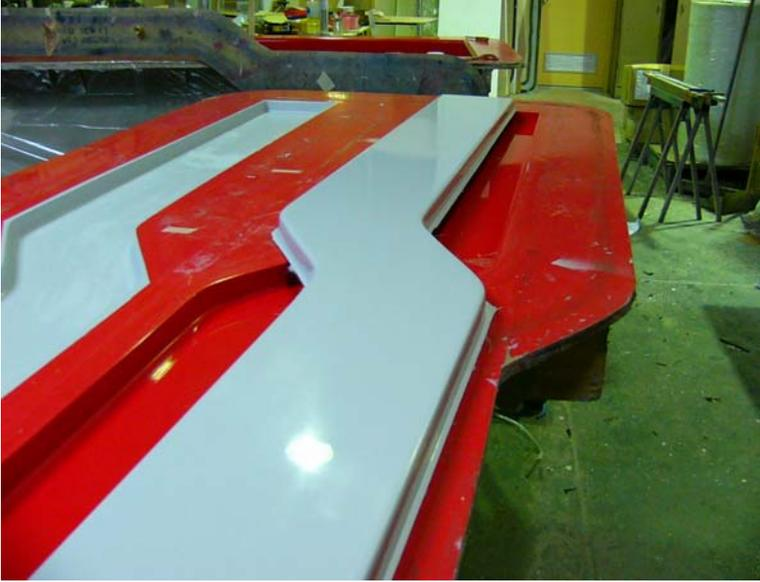
*Figure 8. After curing finished parts are removed and ready to use*
